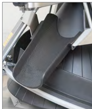
Outfeed chute with small dimples for better outfeed properties.
