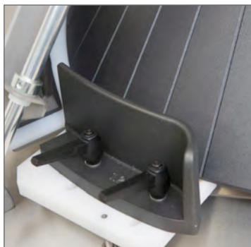
Special designed infeed track, manually adjustable.
